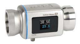
Endress+Hauser Picomag liquid flow meter, magnetic-inductive, 2in female NPT process connection, 0 to 198.1 GPM, 14 to 158 deg F, +/- 3.436E10 liters, 20 to 10,000  $\mu$ S/cm, Output: switch, pulse, analog, discrete input, IO-Link, Output 2: switch, analog, discrete input.
