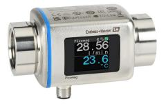
Endress+Hauser Picomag liquid flow meter, magnetic-inductive, 1in female NPT process connection, 0 to 39.6 GPM, 14 to 158 deg F, +/- 3.436E10 liters, 20 to 30,000  $\mu$ S/cm, Output: switch, pulse, analog, discrete input, IO-Link, Output 2: switch, analog, discrete input.
