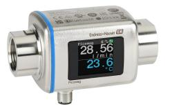
Endress+Hauser Picomag liquid flow meter, magnetic-inductive, 3/4in female NPT process connection, 0 to 19.8 GPM, 14 to 158 deg F, +/- 3.436E10 liters, 20 to  $30,000 \mu$ S/cm, Output: switch, pulse, analog, discrete input, IO-Link, Output 2: switch, analog, discrete input.
