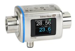
Endress+Hauser Picomag liquid flow meter, magnetic-inductive, 1/2in female NPT process connection, 0 to 9.2 GPM, 14 to 158 deg F, +/- 3.436E10 liters, 20 to 30,000  $\mu$ S/cm, Output: switch, pulse, analog, discrete input, IO-Link, Output 2: switch, analog, discrete input.
