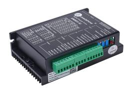
Leadshine DC advanced microstepping stepper drive, 7A per phase, 2-phase output, 24-70 VDC, bipolar, velocity and position mode, 200 to 12800 steps per revolution.
