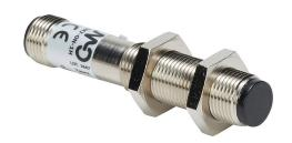
AutomationDirect photoelectric sensor, tubular, threaded, diffuse, infrared, 300mm sensing distance, selectable light-on/dark-on, NPN, teach-in button, 400 Hz switching frequency, metal housing, 4-pin M12 quick-disconnect.
