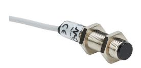
AutomationDirect photoelectric sensor, tubular, threaded, diffuse, infrared, 300mm sensing distance, selectable light-on/dark-on, NPN, teach-in button, 400 Hz switching frequency, metal housing, pigtail.
