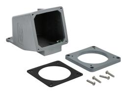
Bryant dead end direct mount back box, (1) 1-1/4in female NPT conduit entries, cast aluminum housing, gray. For use with Bryant 60A devices. AP60 adapter plate and mounting hardware included.
