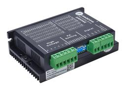
Leadshine DC microstepping stepper drive, 5.6A per phase, 2-phase output, 24-48 VDC, bipolar, position mode, 400 to 25600 steps per revolution.
