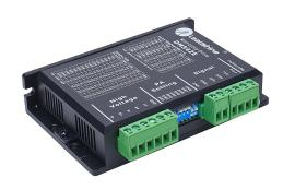
Leadshine DC microstepping stepper drive, 4.2A per phase, 2-phase output, 24-48 VDC, bipolar, position mode, 400 to 25600 steps per revolution.
