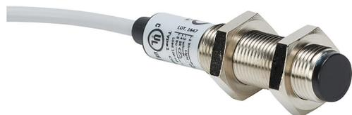
AutomationDirect photoelectric sensor, tubular, threaded, diffuse, infrared light emission, 100mm sensing distance, selectable light-on/dark-on, PNP, teach-in button, 400 Hz switching frequency, metal housing, pigtail.
