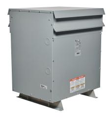
Hammond drive isolation transformer, open core, 220 kVA, 3-phase, 460 VAC Delta primary, 460Y/266 VAC secondary, 60 Hz, NEMA 3R, floor mount.
