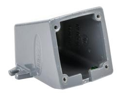
Bryant dead end direct mount back box, (1) 3/4in female NPT conduit entries, cast aluminum housing, gray. For use with Bryant 20A and 30A devices. Mounting hardware included.
