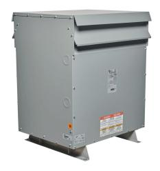
Hammond drive isolation transformer, open core, 175 kVA, 3-phase, 460 VAC Delta primary, 460Y/266 VAC secondary, 60 Hz, NEMA 3R, floor mount.
