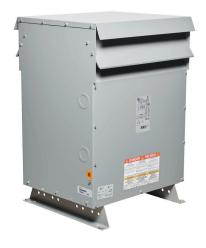
Hammond drive isolation transformer, open core, 93 kVA, 3-phase, 460 VAC Delta primary, 460Y/266 VAC secondary, 60 Hz, NEMA 3R, floor, wall or ceiling mount.
