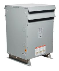
Hammond drive isolation transformer, open core, 75 kVA, 3-phase, 460 VAC Delta primary, 460Y/266 VAC secondary, 60 Hz, NEMA 3R, floor, wall or ceiling mount.
