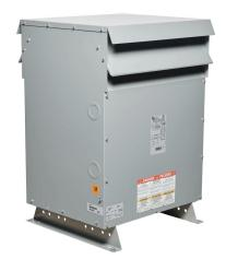
Hammond drive isolation transformer, open core, 63 kVA, 3-phase, 460 VAC Delta primary, 460Y/266 VAC secondary, 60 Hz, NEMA 3R, floor, wall or ceiling mount.
