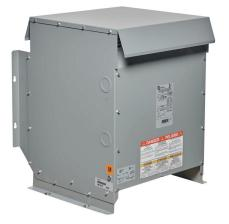
Hammond drive isolation transformer, open core, 51 kVA, 3-phase, 460 VAC Delta primary, 460Y/266 VAC secondary, 60 Hz, NEMA 3R, floor, wall or ceiling mount.
