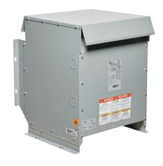
Hammond drive isolation transformer, open core, 34 kVA, 3-phase, 460 VAC Delta primary, 460Y/266 VAC secondary, 60 Hz, NEMA 3R, floor, wall or ceiling mount.
