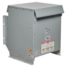
Hammond drive isolation transformer, open core, 20 kVA, 3-phase, 460 VAC Delta primary, 460Y/266 VAC secondary, 60 Hz, NEMA 3R, floor, wall or ceiling mount.
