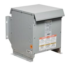
Hammond drive isolation transformer, open core, 11 kVA, 3-phase, 460 VAC Delta primary, 460Y/266 VAC secondary, 60 Hz, NEMA 3R, floor, wall or ceiling mount.
