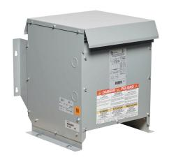
Hammond drive isolation transformer, open core, 7.5 kVA, 3-phase, 460 VAC Delta primary, 460Y/266 VAC secondary, 60 Hz, NEMA 3R, floor, wall or ceiling mount.
