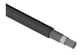
Southwire flexible power cable, unshielded, HDFPC-DLO, RHH/RHW-2 and RW90, single conductor, 8 AWG, tinned copper, EPDM thermoset rubber conductor insulation material, black, CPE thermoset rubber jacket, black, cut to length.
