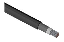
Southwire flexible power cable, unshielded, HDFPC-DLO, RHH/RHW-2 and RW90, single conductor, 6 AWG, tinned copper, EPDM thermoset rubber conductor insulation material, black, CPE thermoset rubber jacket, black, cut to length.
