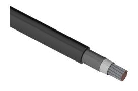
Southwire flexible power cable, unshielded, HDFPC-DLO, RHH/RHW-2 and RW90, single conductor, 4 AWG, tinned copper, EPDM thermoset rubber conductor insulation material, black, CPE thermoset rubber jacket, black, cut to length.
