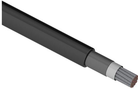
Southwire flexible power cable, unshielded, HDFPC-DLO, RHH/RHW-2 and RW90, single conductor, 4 AWG, tinned copper, EPDM thermoset rubber conductor insulation material, black, CPE thermoset rubber jacket, black, cut to length.
