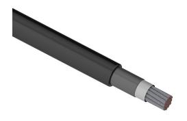
Southwire flexible power cable, unshielded, HDFPC-DLO, RHH/RHW-2 and RW90, single conductor, 4/0 AWG, tinned copper, EPDM thermoset rubber conductor insulation material, black, CPE thermoset rubber jacket, black, cut to length.
