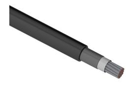
Southwire flexible power cable, unshielded, HDFPC-DLO, RHH/RHW-2 and RW90, single conductor, 3/0 AWG, tinned copper, EPDM thermoset rubber conductor insulation material, black, CPE thermoset rubber jacket, black, cut to length.
