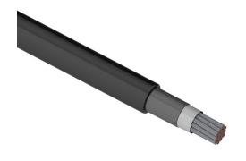
Southwire flexible power cable, unshielded, HDFPC-DLO, RHH/RHW-2 and RW90, single conductor, 3/0 AWG, tinned copper, EPDM thermoset rubber conductor insulation material, black, CPE thermoset rubber jacket, black, cut to length.
