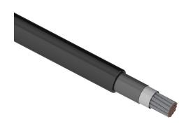
Southwire flexible power cable, unshielded, HDFPC-DLO, RHH/ RHW-2 and RW90, single conductor, 2/0 AWG, tinned copper, EPDM thermoset rubber conductor insulation material, black, CPE thermoset rubber jacket, black, cut to length.
