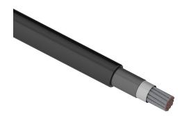
Southwire flexible power cable, unshielded, HDFPC-DLO, RHH/RHW-2 and RW90, single conductor, 1/0 AWG, tinned copper, EPDM thermoset rubber conductor insulation material, black, CPE thermoset rubber jacket, black, cut to length.
