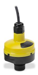
Flowline EchoPod ultrasonic liquid level sensor, 9.8ft/3m sensing range, 4-20 mA and (4) SPST relays, N.O./N.C. selectable, 14-28 VDC operating voltage, 1in male NPT process connection.
