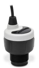
Flowline EchoPod ultrasonic liquid level sensor, 4.1ft/1.25m sensing range, 4-20 mA, 14-28 VDC operating voltage, 1in male NPT process connection.
