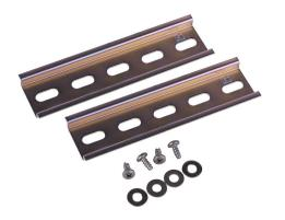
Integra DIN rail, 35mm, 7mm height, 4.9in length, plated steel. Package of 2. For use with 6in wide Impact series polycarbonate enclosures.
