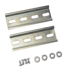
Integra DIN rail, slotted, 35mm, 7mm height, 3.8in length, plated steel. Package of 2. For use with 4in wide Impact series polycarbonate enclosures.
