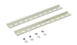
Integra DIN rail, slotted, 35mm, 7mm height, 10.8in length, plated steel. Package of 2. For use with 12in wide Premium series polycarbonate enclosures.
