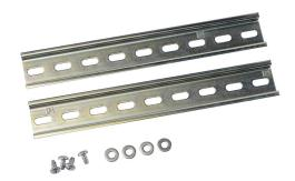
Integra DIN rail, slotted, 35mm, 7mm height, 8.8in length, plated steel. Package of 2. For use with 10in wide Premium series polycarbonate enclosures.
