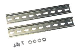
Integra DIN rail, slotted, 35mm width, 7mm height, 8.8in length, plated steel. Package of 2. For use with 10in wide Premium series polycarbonate enclosures.
