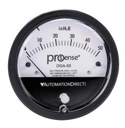
ProSense differential pressure gauge, 4in dial diameter, 0 to 50.0in of water column, black die-cast aluminum case, aluminum and silicone rubber wetted parts, (2) high and (2) low 1/8in female NPT process connection, panel or surface mount.
