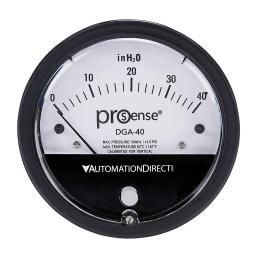
ProSense differential pressure gauge, 4in dial diameter, 0 to 40.0in of water column, black die-cast aluminum case, aluminum and silicone rubber wetted parts, (2) high and (2) low 1/8in female NPT process connection, panel or surface mount.
