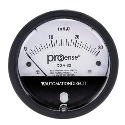
ProSense differential pressure gauge, 4in dial diameter, 0 to 30.0in of water column, black die-cast aluminum case, aluminum and silicone rubber wetted parts, (2) high and (2) low 1/8in female NPT process connection, panel or surface mount.
