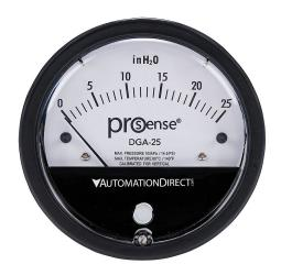
ProSense differential pressure gauge, 4in dial diameter, 0 to 25.0in of water column, black die-cast aluminum case, aluminum and silicone rubber wetted parts, (2) high and (2) low 1/8in female NPT process connection, panel or surface mount.
