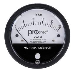
ProSense differential pressure gauge, 4in dial diameter, 0 to 25.0in of water column, black die-cast aluminum case, aluminum and silicone rubber wetted parts, (2) high and (2) low 1/8in female NPT process connection, panel or surface mount.
