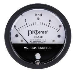
ProSense differential pressure gauge, 4in dial diameter, 0 to 20.0in of water column, black die-cast aluminum case, aluminum and silicone rubber wetted parts, (2) high and (2) low 1/8in female NPT process connection, panel or surface mount.
