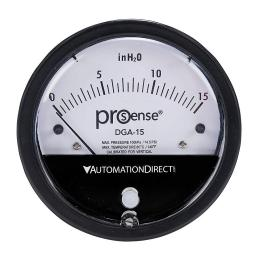
ProSense differential pressure gauge, 4in dial diameter, 0 to 15.0in of water column, black die-cast aluminum case, aluminum and silicone rubber wetted parts, (2) high and (2) low 1/8in female NPT process connection, panel or surface mount.
