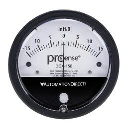
ProSense differential pressure gauge, 4in dial diameter, -15.0 to +15.0in of water column, black die-cast aluminum case, aluminum and silicone rubber wetted parts, (2) high and (2) low 1/8in female NPT process connection, panel or surface mount.
