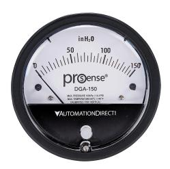
ProSense differential pressure gauge, 4in dial diameter, 0 to 150.0in of water column, black die-cast aluminum case, aluminum and silicone rubber wetted parts, (2) high and (2) low 1/8in female NPT process connection, panel or surface mount.
