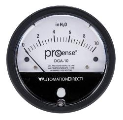
ProSense differential pressure gauge, 4in dial diameter, 0 to 10.0in of water column, black die-cast aluminum case, aluminum and silicone rubber wetted parts, (2) high and (2) low 1/8in female NPT process connection, panel or surface mount.
