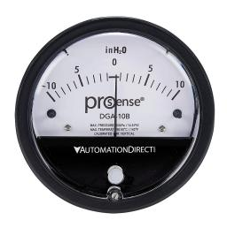
ProSense differential pressure gauge, 4in dial diameter, -10.0 to +10.0in of water column, black die-cast aluminum case, aluminum and silicone rubber wetted parts, (2) high and (2) low 1/8in female NPT process connection, panel or surface mount.
