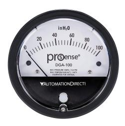
ProSense differential pressure gauge, 4in dial diameter, 0 to 100.0in of water column, black die-cast aluminum case, aluminum and silicone rubber wetted parts, (2) high and (2) low 1/8in female NPT process connection, panel or surface mount.
