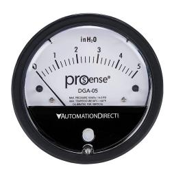
ProSense differential pressure gauge, 4in dial diameter, 0 to 5.0in of water column, black die-cast aluminum case, aluminum and silicone rubber wetted parts, (2) high and (2) low 1/8in female NPT process connection, panel or surface mount.
