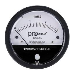
ProSense differential pressure gauge, 4in dial diameter, 0 to 3.0in of water column, black die-cast aluminum case, aluminum and silicone rubber wetted parts, (2) high and (2) low 1/8in female NPT process connection, panel or surface mount.
