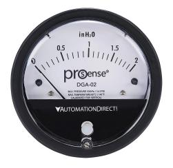
ProSense differential pressure gauge, 4in dial diameter, 0 to 2.0in of water column, black die-cast aluminum case, aluminum and silicone rubber wetted parts, (2) high and (2) low 1/8in female NPT process connection, panel or surface mount.
