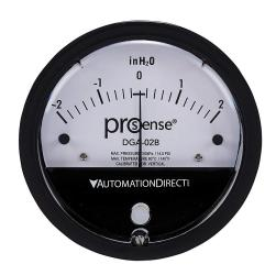
ProSense differential pressure gauge, 4in dial diameter, -2.0 to +2.0in of water column, black die-cast aluminum case, aluminum and silicone rubber wetted parts, (2) high and (2) low 1/8in female NPT process connection, panel or surface mount.
